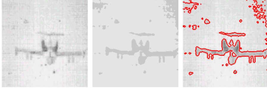
Figure 11: Left: an original grayscale image of an airplane. Middle: a weighted-CVT-based segmentation into two segments (with weights \lambda_\ell = |U_\ell| , i.e., \alpha = 1 ) and with subsequent averaging (with \sigma = 1.5 and \beta = 0.05 ). Right: the corresponding edges superimposed on the original image.
