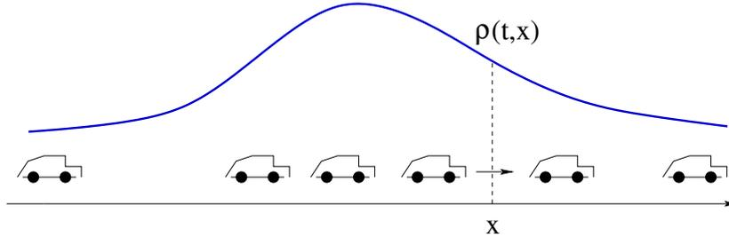
Figure 1: Modeling traffic flow by a PDE. Here  $\rho$  is the density of cars, whice the product  $\rho \cdot v(\rho)$  gives the flux of cars.
